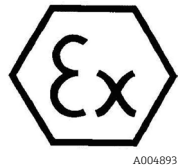
Figure 3. ATEX label for use in hazardous areas
