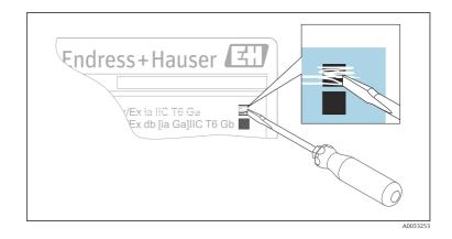
Depending on the type of protection used: Observe the safety instructions for installation with explosion protection "Intrinsic safety Ex ia", "Flameproof enclosure Ex db" or "Equipment dust ignition protection by enclosure Ex t".
