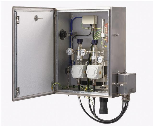
PRS within an heated SS316 enclosure including two heated pressure regulators, isolated valves, pressure safety valves and sleeve for a heated traced line
