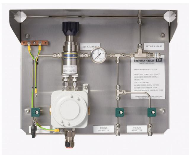
Natural gas PRS on a Sunshade SS316 plate, including one heated pressure reducer, inlet on/off valve and a pressure safety valves
