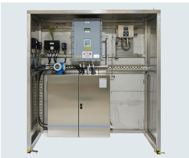
Biomethane quality control complete shelter solution with a trace H<sub>2</sub>S analyzer (SS2100i-1), a moisture analyzer (J22), and an oxygen analyzer (OXY5500). This solution benefits from a centralized power switch, electrical and signal distribution, as well as a cabinet for sample conditioning.
