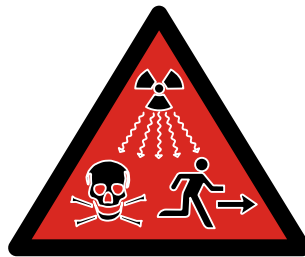
Warning symbol for highly radioactive source according to ISO21482
