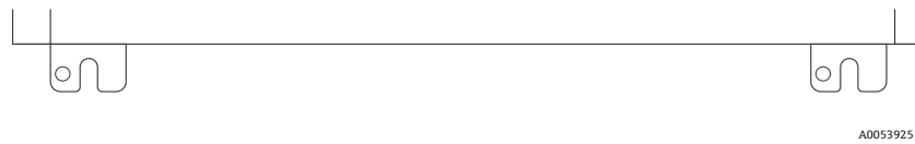
Figure 8. Slotted bottom mounting tabs of enclosure
