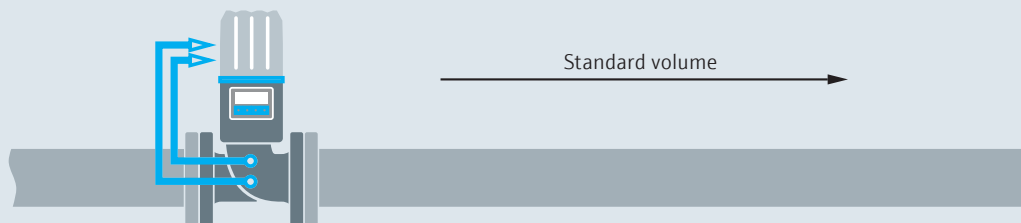
Gas flow meter with volume corrector and external p/T sensor
