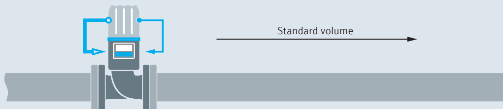
Gas flow meter with volume corrector and internal p/T sensor
