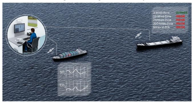
The MARSIC series of ship emissions measuring devices give ship operators the safety they need. In combination with the appropriate software, MARSIC generates an emissions profile that can be linked with the current ship location. This provides enormous added value: the ship's crew can initiate the necessary measures immediately on entering an Emission Control Area (ECA).
