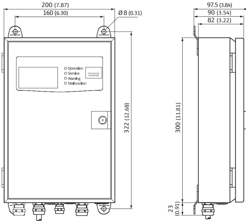
GM35 AWE evaluation unit: cast metal enclosure (dimensions in mm (inch))
