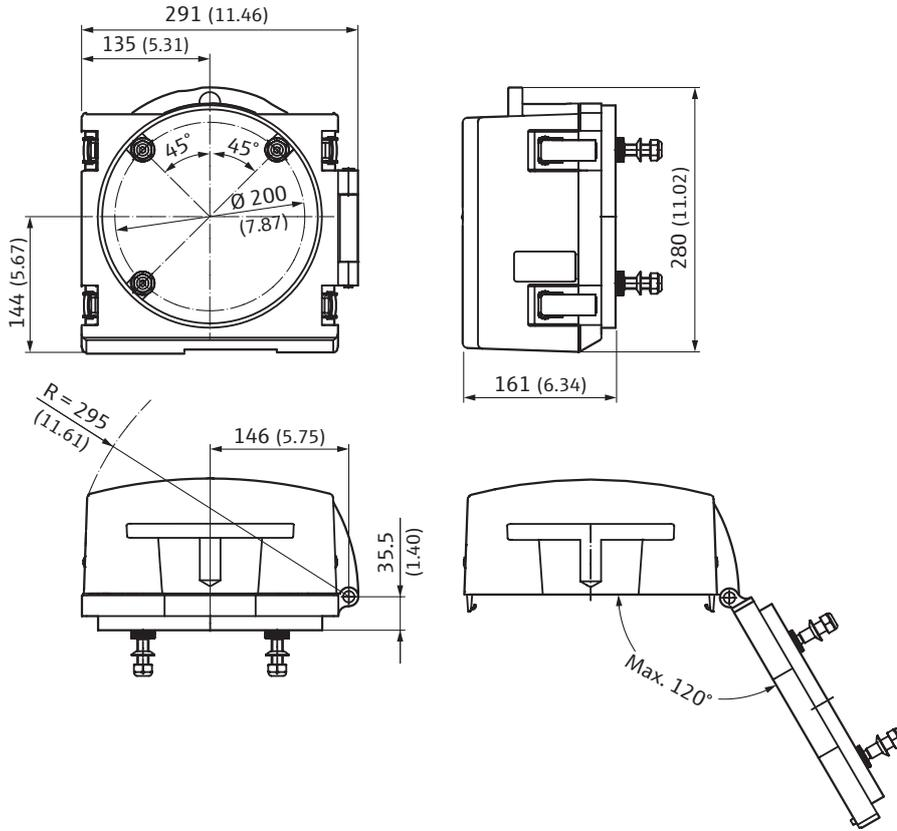
GM35 AWE evaluation unit: steel sheet enclosure (dimensions in mm (inch))
