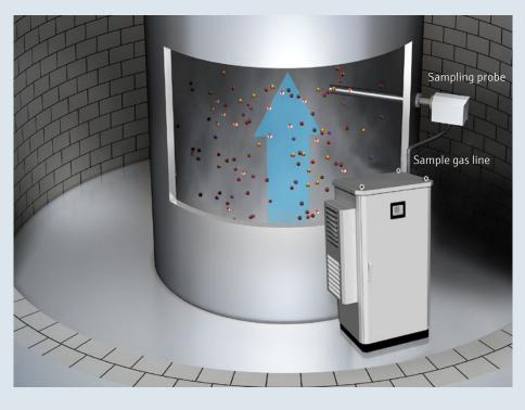
MERCEM300Z measures hot extractive: The flue gas is extracted with a sampling probe and transported to the analyzer via a sample gas line. All components having contact with the sample gas, such as probe, sample gas line and converter in the analyzer, are heated to such a high temperature that no adsorption and no elution occur.
