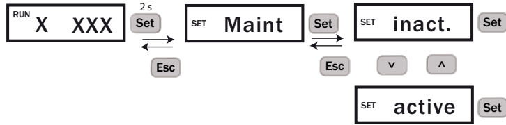
Fig. 38: Activating the setting range via menu item "Maint"
