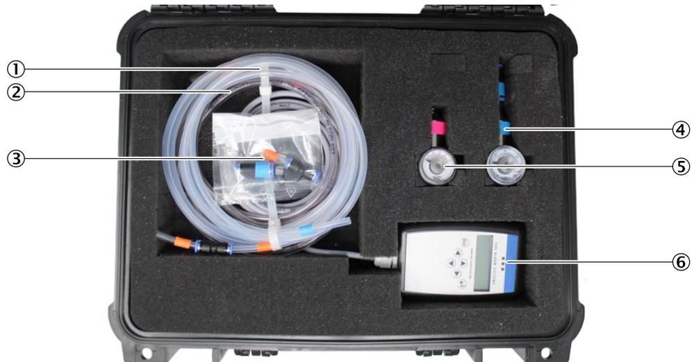
Fig. 2: Contents, Gas Adjustment Kit
