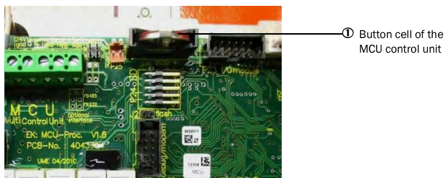
Fig. 53: Button cell exchange, MCU
