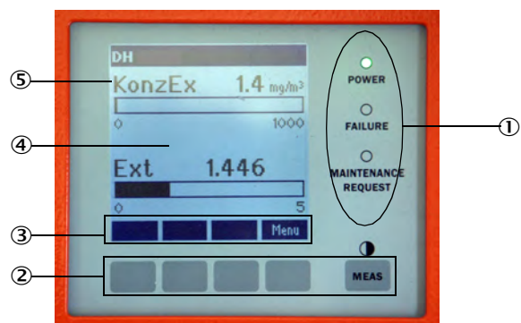
Fig. 50: Functional elements LC display of MCU control unit
