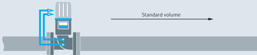
Gas flowmeter with volume corrector and external p/T sensor
