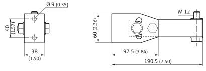
Connection unit, aluminum housing version (dimensions in mm (inch))
