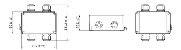
Connection unit, stainless steel housing version (dimensions in mm (inch))
