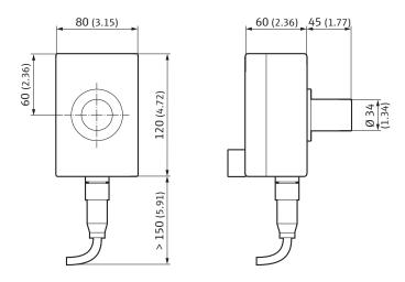
FLSE200-H and FLSE200-HM sender/receiver units (dimensions in mm (inch))
