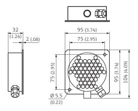
Cover for connections; with air inlet at the side (dimensions in mm (inch))
