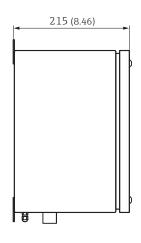
MCU-N control unit; wall-mounting enclosure, compact version (for non-hazardous areas only) (dimensions in mm (inch))
