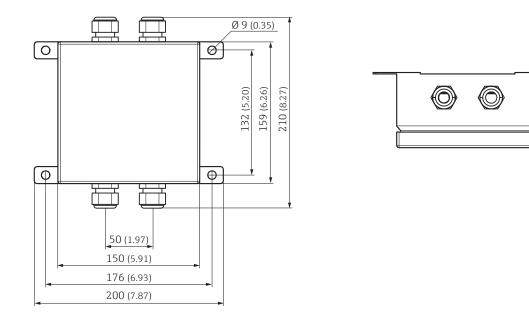
Air inlet with protective grading for wall mounting (dimensions in mm (inch))
