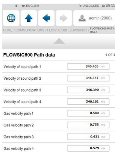
Fig. 31: Menu item “Communication/Flowsic600-XT Flow Meter/Flowsic600-XT Path Data”
