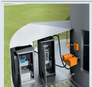
The MCS100FT can continuously measure the following components using one single extractive heated gas sample: HCl, CO, NO $_{\rm x}$  as the sum of NO and NO $_{\rm 2}$ , SO $_{\rm 2}$ , NH $_{\rm 3}$ , O $_{\rm 2}$ , H $_{\rm 2}$ O, CO $_{\rm 2}$ , C $_{\rm ges}$ , and HF. For normalization, pressure and temperature parameters are also measured. The QAL3 test can be carried out without test gas with the certified, integrated filter.
