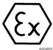
Figure 3. ATEX label for use in hazardous areas
