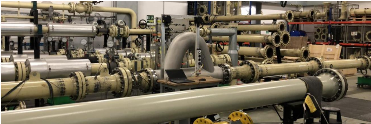
Figure 3: Proline Promass Q DN200 being calibrated in Pigsar facilities using natural gas as calibration fluid.
