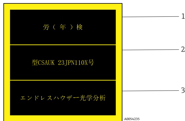
Figure 7. JPEX label for use in hazardous areas
