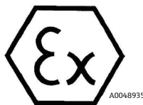
Figure 5. ATEX label for use in hazardous areas
