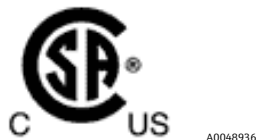
Figure 4. Label showing equipment is approved for use in hazardous areas in the United States and Canada
