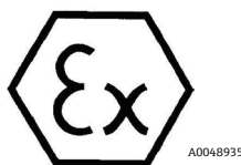
Figure 6. ATEX label for use in hazardous areas
