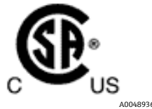
Figure 3. Label showing equipment is approved for use in hazardous areas in the United States and Canada
