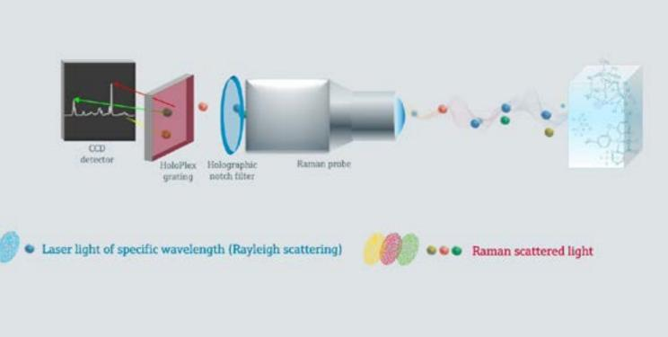
The collected light is interpreted as a spectrum by the camera, creating a "molecular fingerprint" of the material being sampled.
