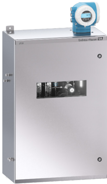
Figure 2: The Endress+Hauser JT33 TDLAS gas analyzer uses a differential spectroscopy technique to quantify low ppb to ppm levels of H 2 S in the outlet gas stream of an amine treatment unit.
