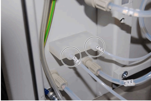
39 Coupling with short thread \frac{1}{8}'' \times 28\text{UNF} on condensate drain adapter for acid supply
