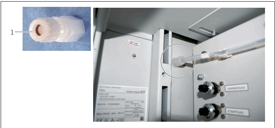
18 Installation position of the bulkhead coupling
