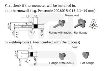
In case of installation in a thermowell:
