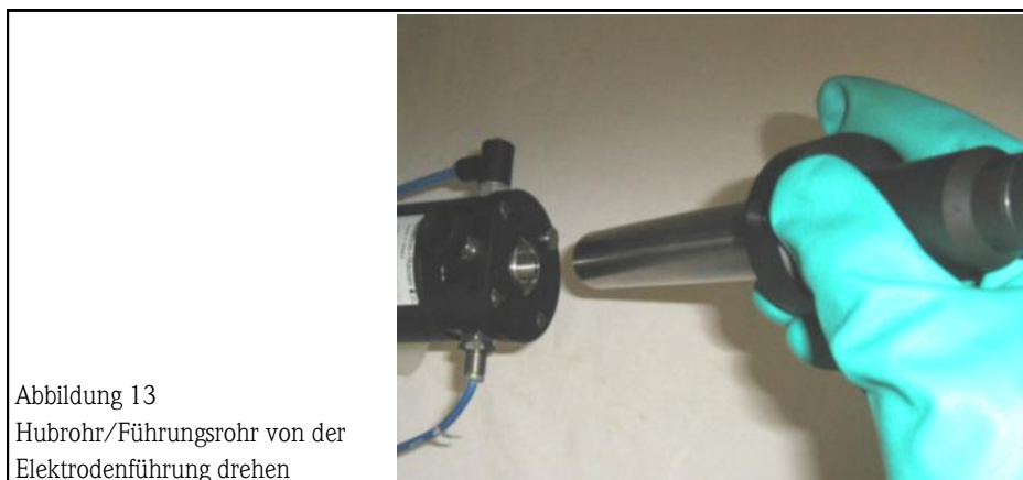
Figure 13 Turn the retractable pipe/guide pipe from the electrode guide
