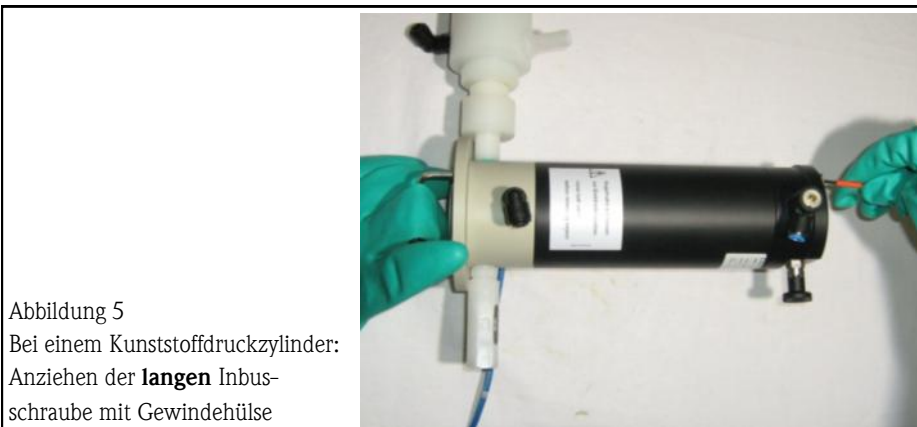
Figure 5 At a plastic pressure actuator: Tighten the long Allen screw with the threaded sleeve
