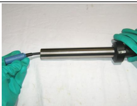
Figure 5 Push the Memosens cable into the protective pipe
