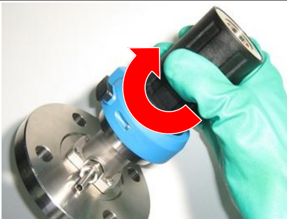
Figure 29 Turn the immersion pipe into the measurement position
