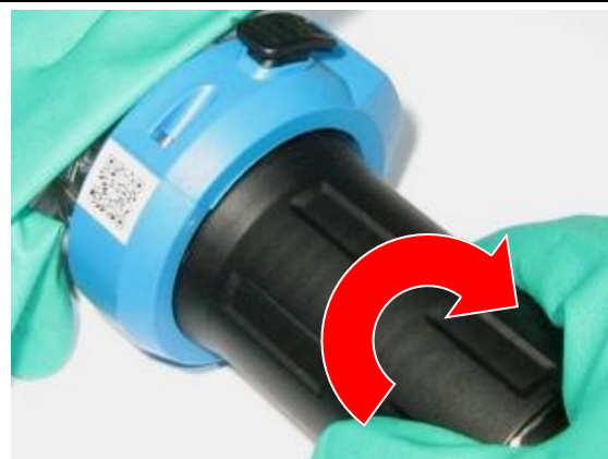
Figure 17 Move the retractable pipe/guide pipe to the measurement position
