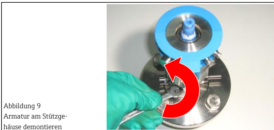
Figure 9 Demount the process assembly at the support housing
