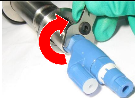
Figure 10 Turn the KCl electrode/sensor into the electrode guide
