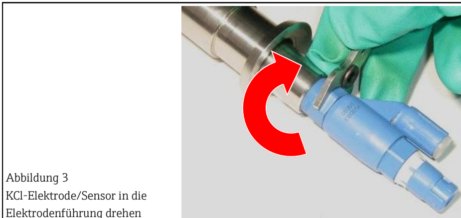
Figure 3 Turn the KCl electrode/sensor into the electrode guide
