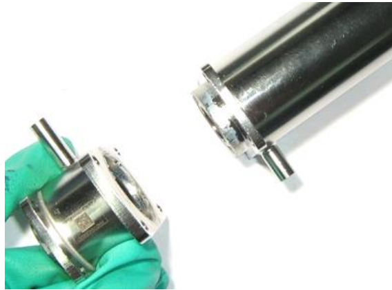
Figure 7 Separate the service chamber from the pre chamber
