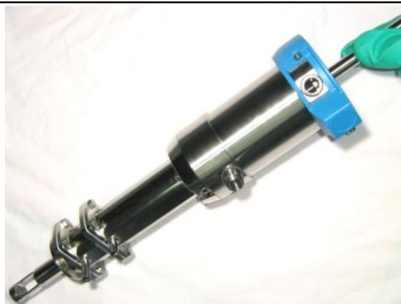
Figure 26 Push the immersion pipe into the measurement position
