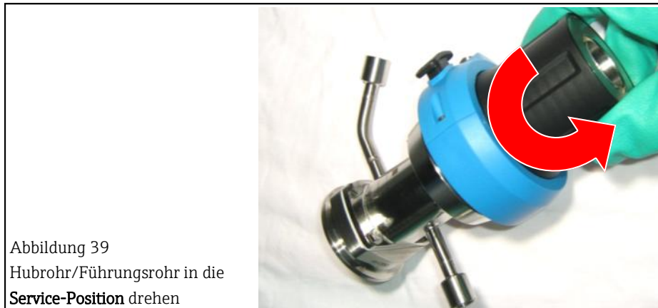
Figure 39 Turn the retractable pipe/guide pipe into the service position
