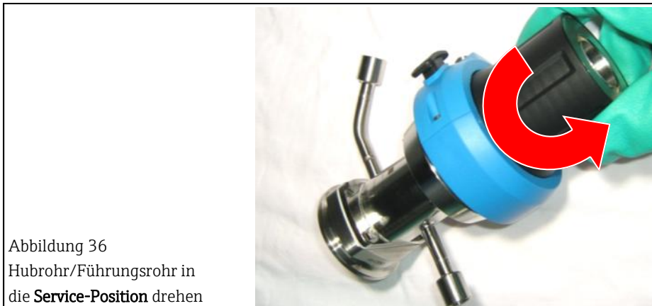
Figure 36 Turn the retractable pipe/guide pipe into the service position
