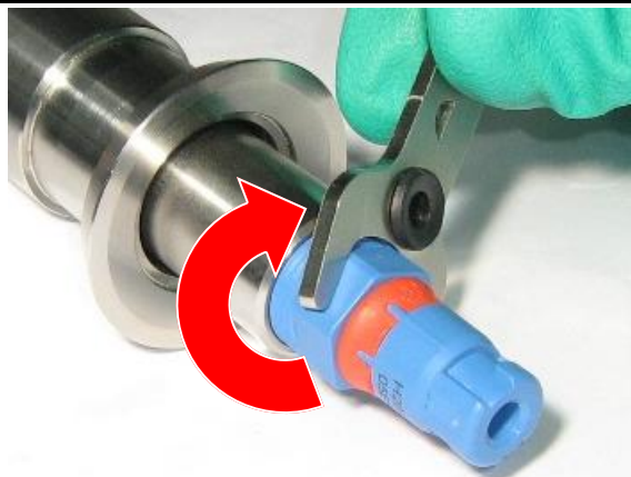
Figure 13 Turn the new electrode/sensor into the electrode guide
