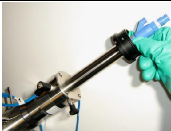
Figure 7 Turn the KCl electrode/sensor into the electrode guide
