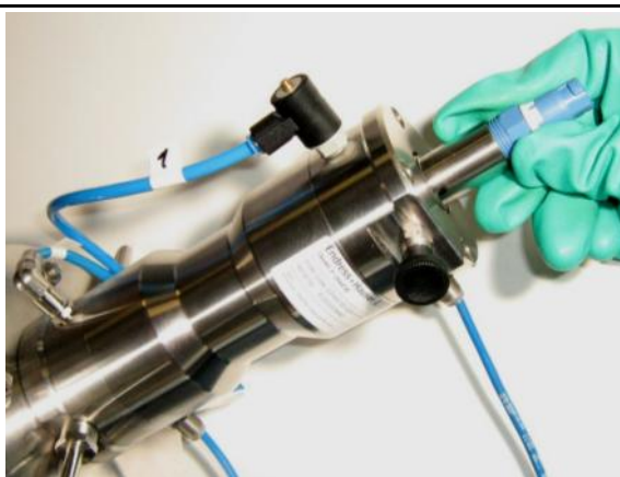
Figure 5 Turn the KCl electrode/sensor into the electrode guide
