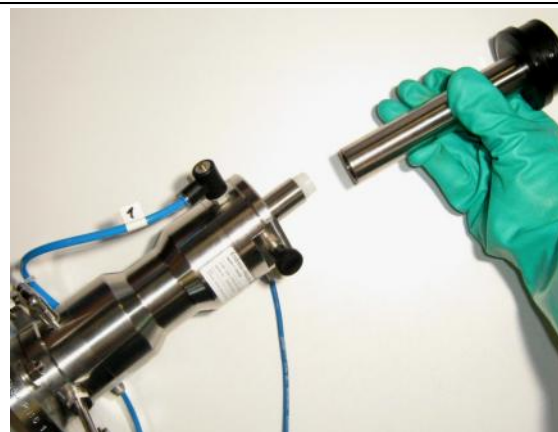
Figure 3 Turn the KCl retractable pipe/guide pipe from the electrode guide
