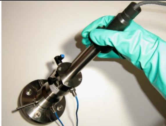
Figure 4 Turn the retractable pipe/guide pipe on the electrode guide
