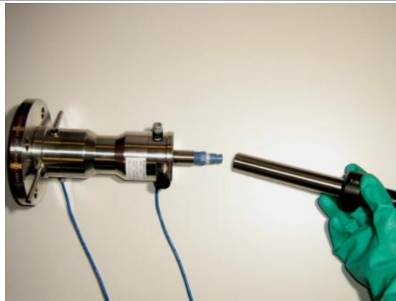
Figure 2 Turn the retractable pipe/guide pipe from the electrode guide
