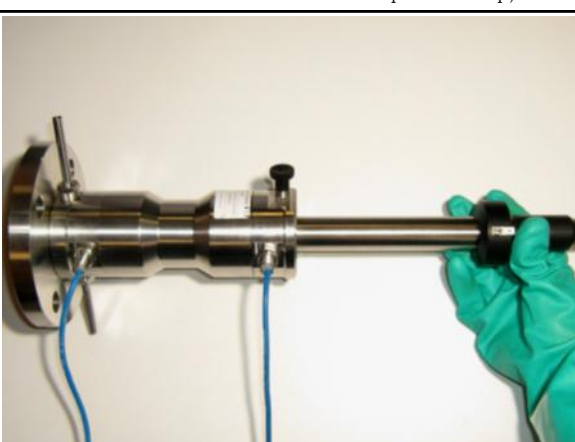
Figure 19 Pull the retractable pipe/guide pipe into the service position
