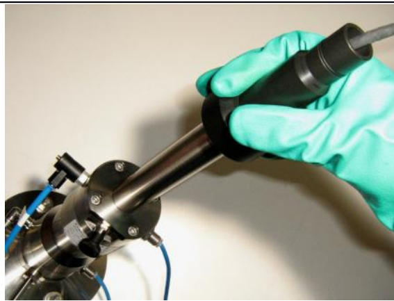
Figure 5 Turn the retractable pipe/guide pipe on the electrode guide
