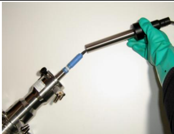
Figure 6 Turn the retractable pipe/guide pipe from the electrode guide
