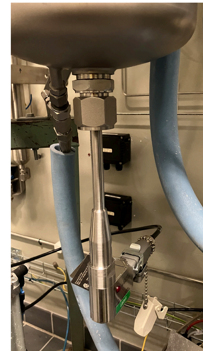
The Raman probes were immersed in a lab-scale reactor designed for future upscaling to the pilot plant. With a 10m fiber cable, the Raman probes were connected to the Raman analyzer located in a controlled room.
