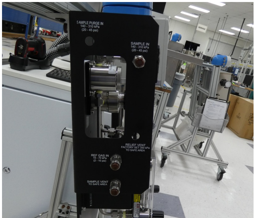
Figure 1 - The validation or reference gas bulkhead port is found near the sample inlet port on most analyzers.
