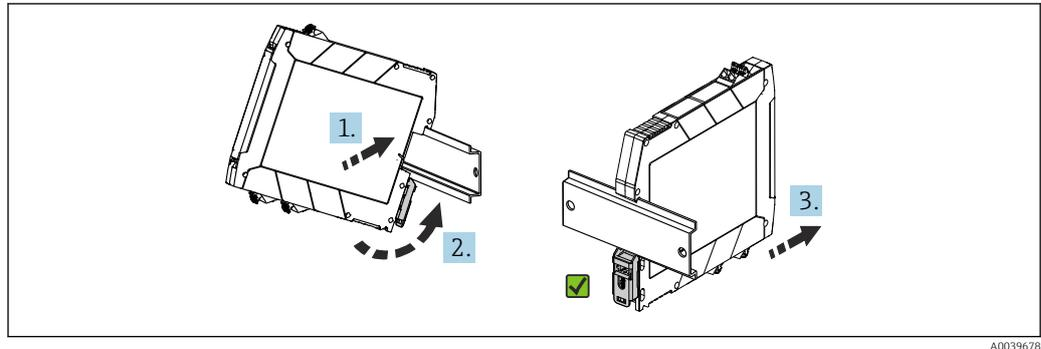
3 Montage Hutschienentransmitter
