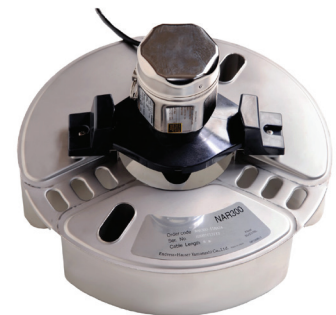
Figure 5: The Endress+Hauser Model NAR300 leak detection switch combines vibration and conductivity detection to provide indication of conductive and nonconductive liquids
