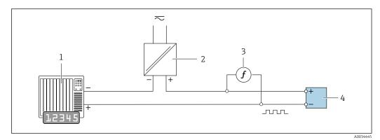
■ 9 External verification of passive pulse/frequency output
