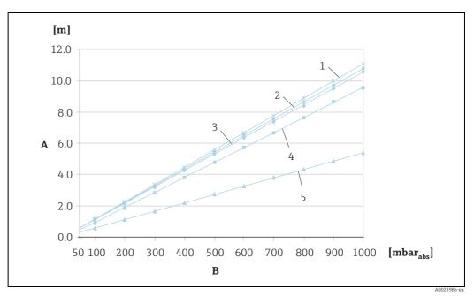
The maximum height difference depends on the density of the filling oil and the smallest ever pressure that is permitted to occur at the diaphragm seal (empty vessel), see illustration below:
