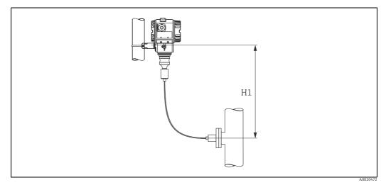
Fig. 10: Installation above the lower diaphragm seal
