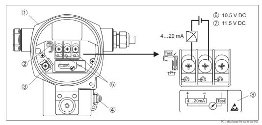
Fig. 18: Electrical connection 4 to 20 mA HART. Observe also  $\rightarrow \square 28$ , "Supply voltage".
