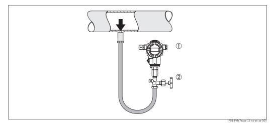
Fig. 8: Measuring arrangement for pressure measurement in liquids
