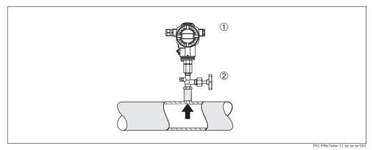
Fig. 6: Measuring arrangement for pressure measurement in gases
