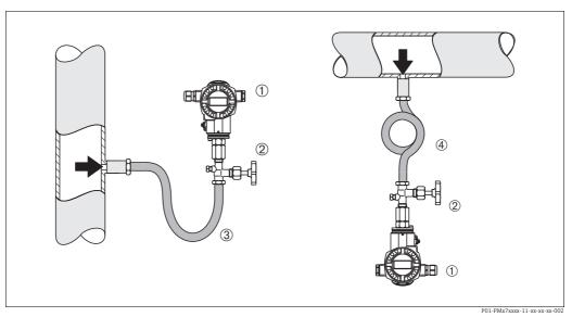
Fig. 7: Measuring arrangement for pressure measurement in steams
