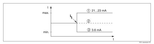
*Fig. 26: Current output in the event of an alarm*
