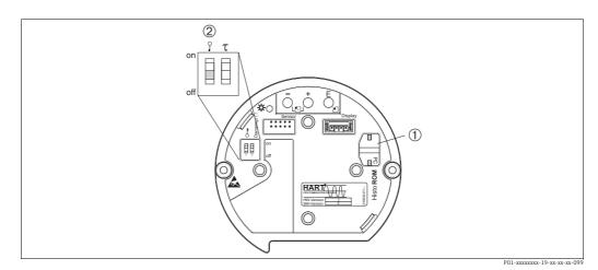
Abb. 24: Electronic insert with optional HistoROM<sup>®</sup>/M-DAT memory module
