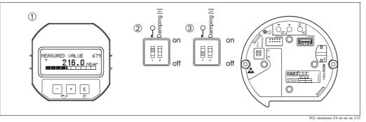
Fig. 25: DIP-switch position "Hardware locking" on the electronic insert
