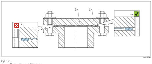
1 Process isolating diaphragm 2 Seal
