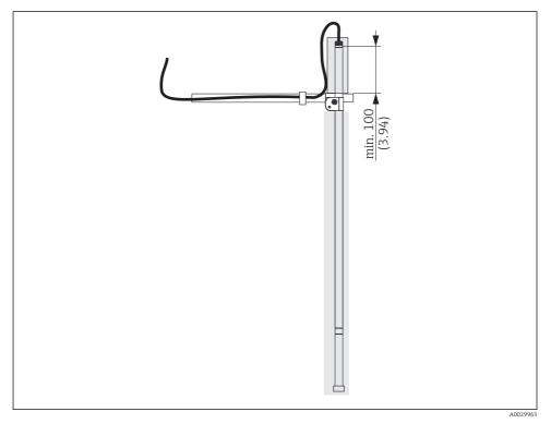
■ 9 Retaining point (shown without splash protection cap)
