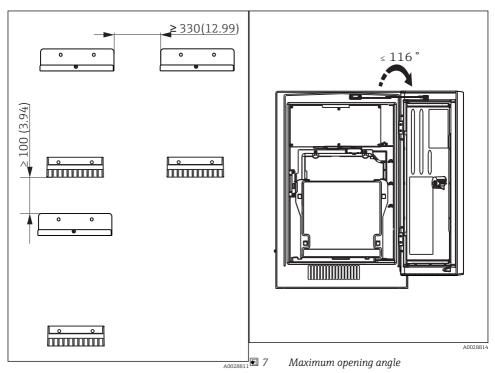
■ 6 Minimum spacing required for mounting.Engineering unit mm (in).
