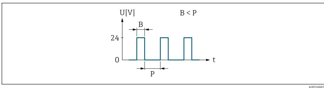
5 Quantity-proportional pulse (pulse value) with pulse width to be configured
