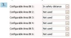
Select one of these bits (in the example: Configurable Area Bit 1) and select **In safety distance** from the associated drop-down menu. Confirm the selection by pressing the Enter key.
