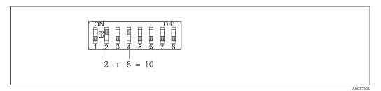
$\blacksquare$  22 Example of hardware addressing: switch 8 is in position "OFF"; switches 1 to 7 define the address.
