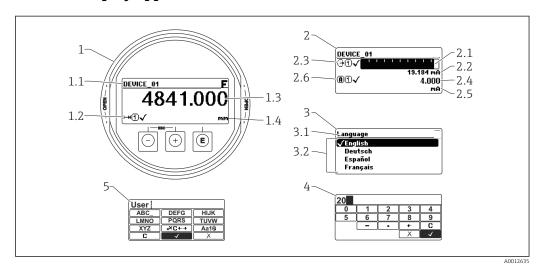
■ 20 Appearance of the display and operation module for on-site operation
