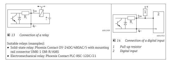
For optimum interference immunity we recommend to connect an external resistor (internal resistance of the relay or Pull-up resistor) of  $< 1000 \Omega$ .
