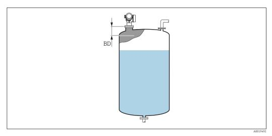
₹ 34 Blocking distance (BD) for liquid measurements
