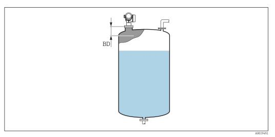
■ 38 Blocking distance (BD) for liquid measurements
