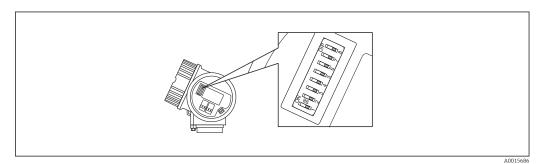
■ 21 Address switches in terminal compartment
