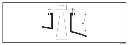
■ 6 Nozzle height for horn antenna (FMR51)
