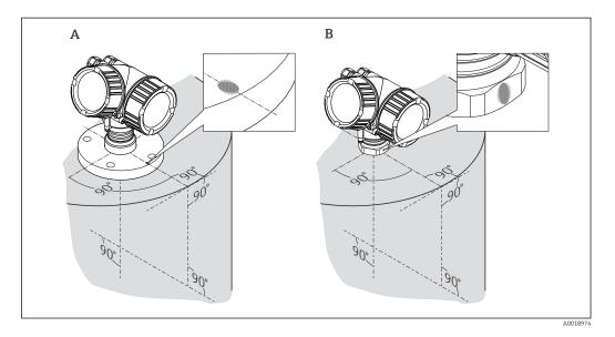
Depending on the device version the marking may be a circle or two short parallel lines.
