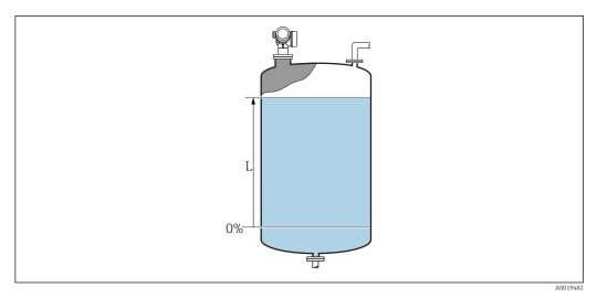
■ 32 Level in case of liquid measurements
