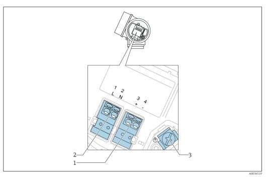
$\blacksquare$  10 Terminal assignment 4-wire: 4-20 mA HART (90 to 253  $V_{AC}$ )
