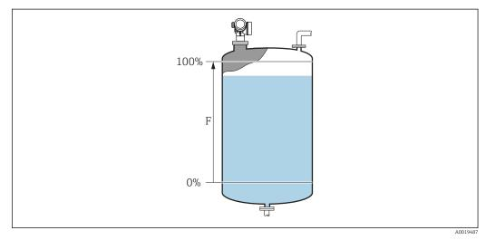
$\blacksquare$  31 Full calibration (F) for level measurements in liquids
