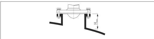
■ 7 Nozzle height for horn antenna, flush mount (FMR52)
