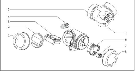
**₽** 3 Design of the electronics housing
