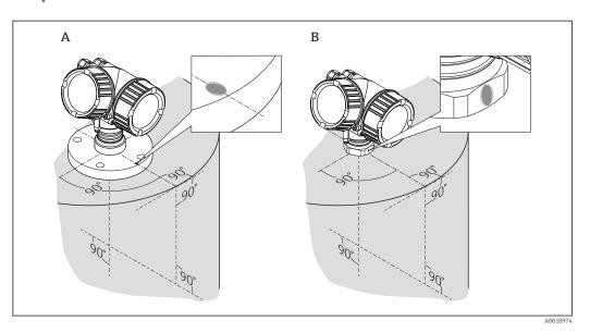
Depending on the device version the marking may be a circle or two short parallel lines.
