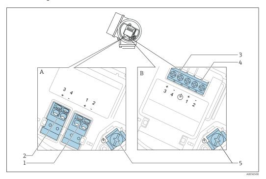
$\blacksquare 11$  Terminal assignment PROFIBUS PA / FOUNDATION Fieldbus
