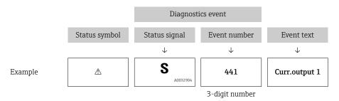
If two or more diagnostic messages are pending simultaneously, only the message with the highest priority is shown. Additional pending diagnostic messages can be shown in the **Diagnostic list** submenu.
