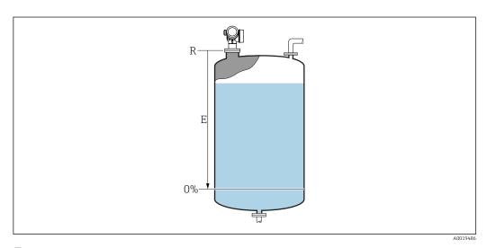
$\blacksquare$  30 Empty calibration (E) for level measurements in liquids
