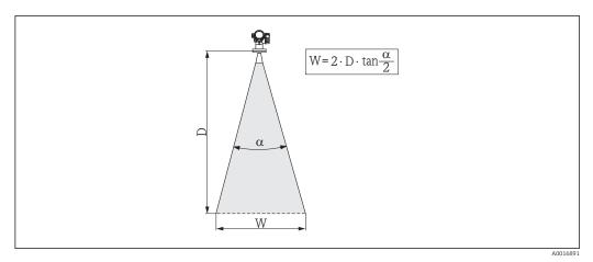
$\blacksquare$  5 Relationship between beam angle  $\alpha$ , distance D and beamwidth diameter W
