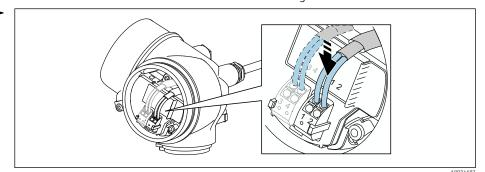
6. If using shielded cables: Connect the cable shield to the ground terminal.
