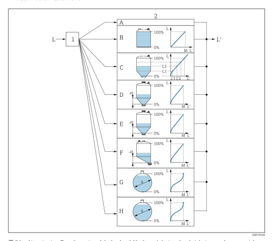
₹ 36 Linearization: Transformation of the level and (if relevant) the interface height into a volume or weight; the transformation is dependent on the shape of the vessel.
