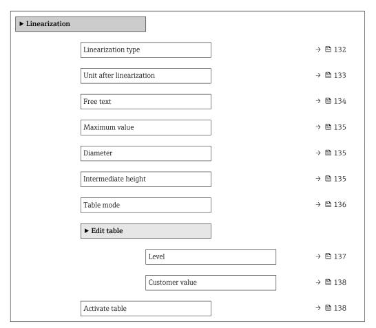
Structure of the submenu in an operating tool (e.g. FieldCare)
