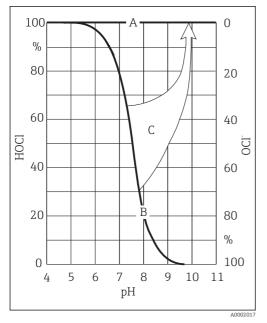
Without pH compensation, the chlorine measuring system must be recalibrated when the pH value changes.
