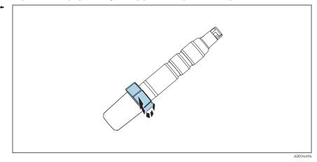
9 Securing protection cap by rotating the top part
