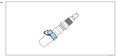
☑ 5 Releasing top part of protection cap by turning
