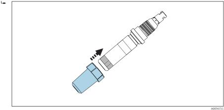
• 8 Carefully slide protection cap onto the membrane cap.
