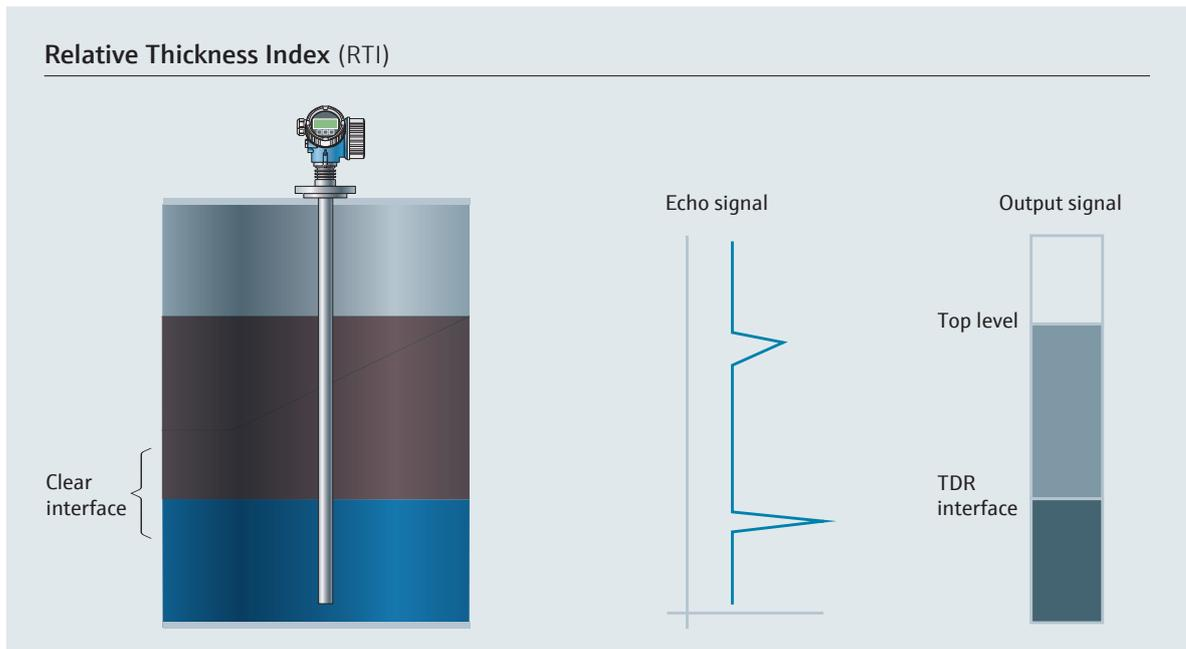
At a clean interface of water and condensate the Relative Interface Echo Amplitude is higher than 70mV.
