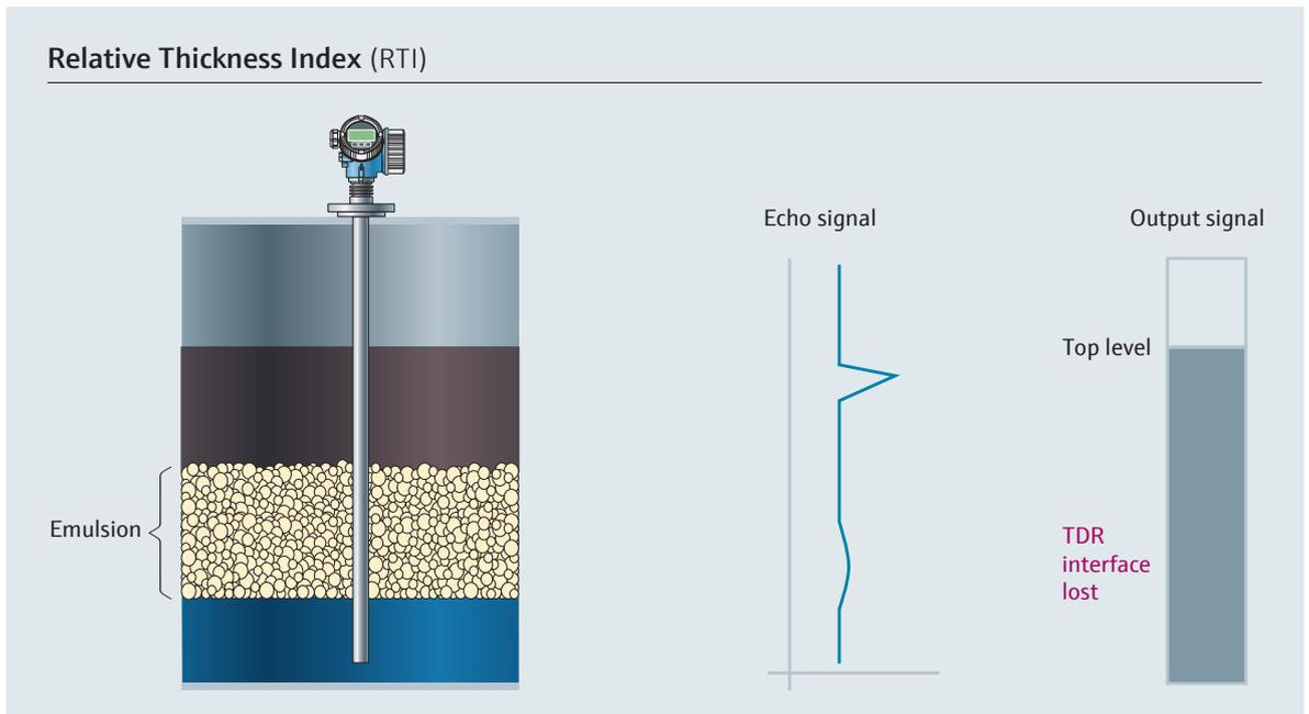
What they found was a Relative Echo Amplitude dropping to around 30mV (Relative Thickness Index 30) as soon as emulsion occurred. The emulsion was about 25-50mm. As the emulsion is getting thicker to about 80-100 mm (RTI of 10 or less) the Relative Interface Echo Amplitude drops further. Even when they lost the Relative Interface Echo altogether (0mV) the instrument FMP55 still measured with the capacitance probe.
