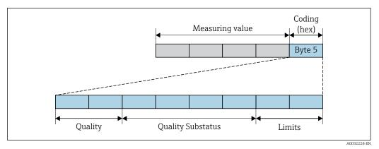
■ 28 Structure of the coding byte
