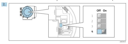
To switch addressing from software addressing to hardware addressing: set the DIP switch to  $\mathbf{On}$ .
