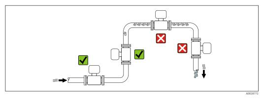
To prevent measuring errors arising from accumulation of gas bubbles in the measuring tube, avoid the following mounting locations in the pipe:
