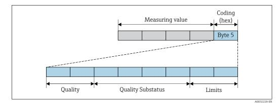
■ 28 Structure of the coding byte
