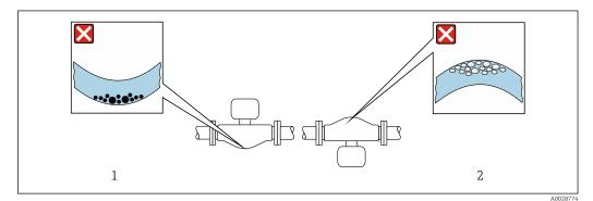
☑ 5 Orientation of sensor with curved measuring tube
