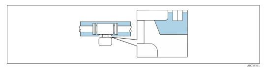
Image: Thermal insulation with extended neck free
