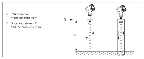
Figure 2: FMCW principle: Emission and reflection of the continuous wave
