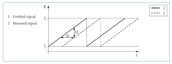
Figure 3: FMCW principle: Results of the frequency modulation
