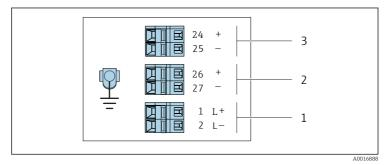
I Terminal assignment 4-20 mA HART with pulse/frequency/switch output
