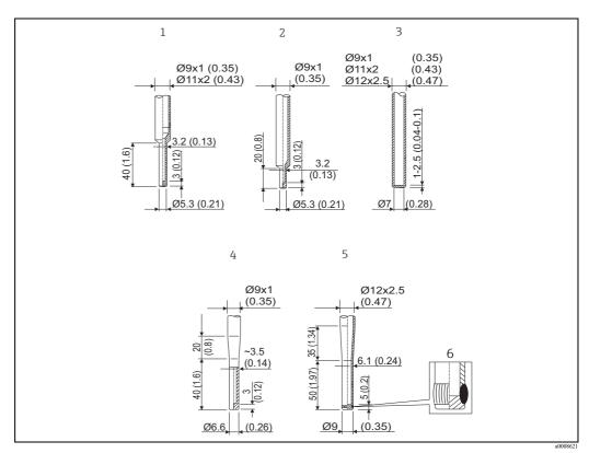
Available versions of thermowell tips (reduced, straight, tapered). Maximum surface roughness  $\leq$  Ra 0.8  $\mu$ m (31.5  $\mu$ in)
