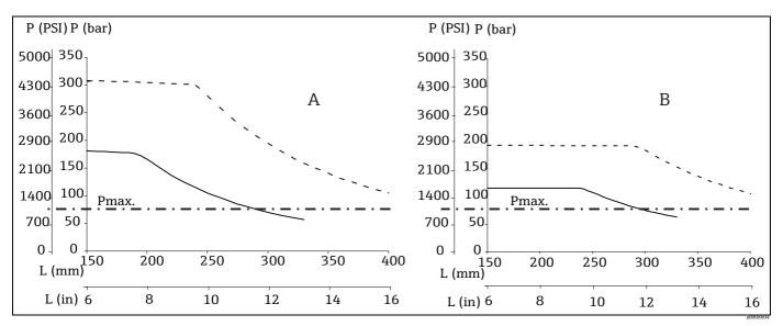
Maximum permitted process pressure for tube diameter, limited to 75 bar (1088 psi) by the threaded process connection – Thermowell diameter 9 x 1 mm (0.35 in) ------
