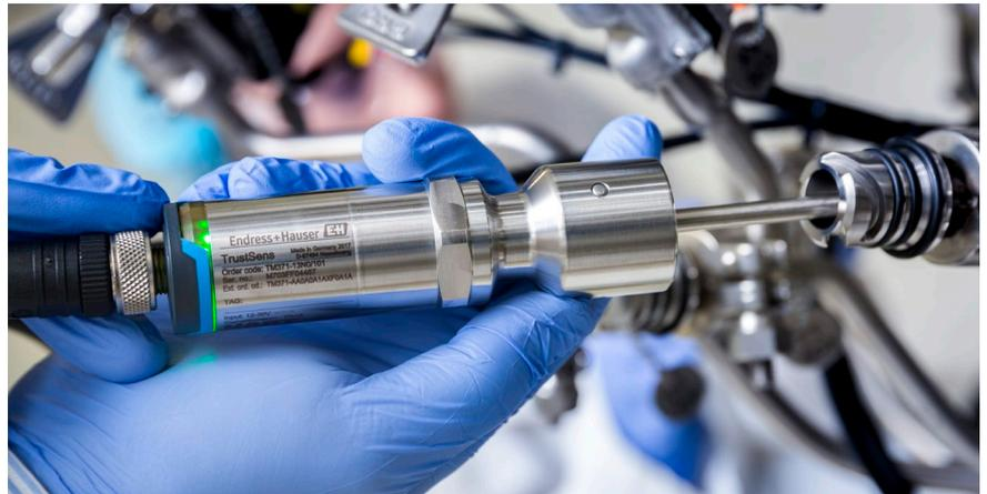
Temperature measurement instruments are widely used in pharmaceutical processes as sufficiently high temperatures must be guaranteed in all system units during the sterilization phase to ensure that all germs are killed off. The accuracy of these measurements must be verified with the help of regular sensor calibrations, since incorrect measurements can pose a hygiene risk. New technology of inline self-calibrating thermometers can contribute to minimizing the risk of incorrect measurements.
