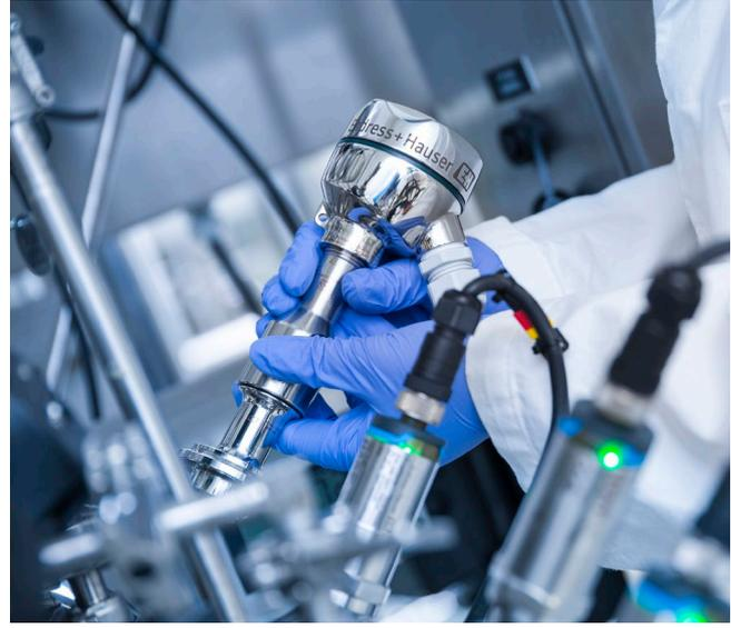
Common setup for an on-site manual calibration procedure using a block calibrator
