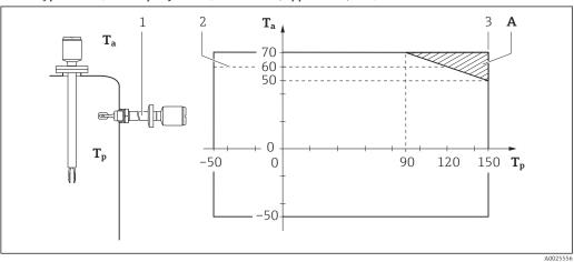
Device type FTL80, FTL81, Basic specification, Position 7 (Application) = A, B Device type FTL85, Basic specification, Position 7 (Application) = P, T
