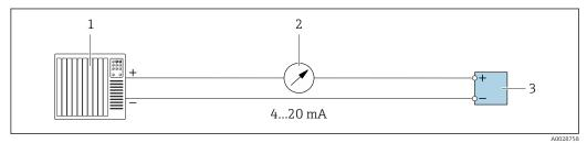
Connection example for current output, active, 4 to 20
