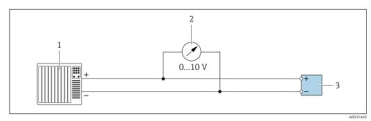
■ 10 Connection example for voltage output, active, 0 to 10 V
